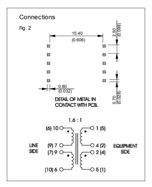
Dimensions shown are in millimetres (inches). Terminal references in parentheses denote alternative customer designation.
